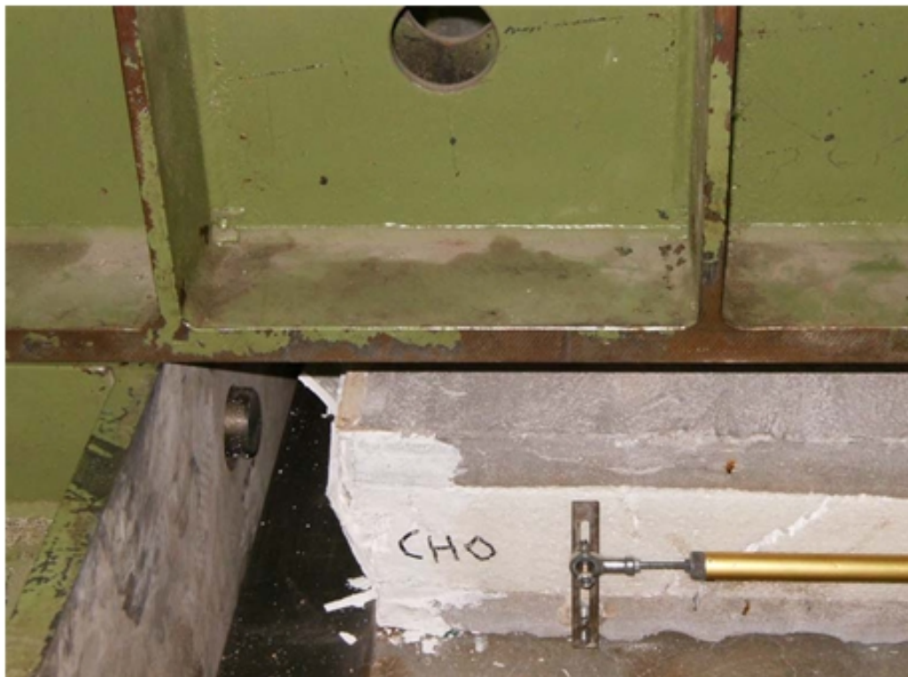
Figure 22: Sliding of the polystyrene slab
