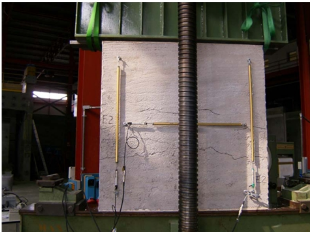
Figure 21: Fissure summary during testing
