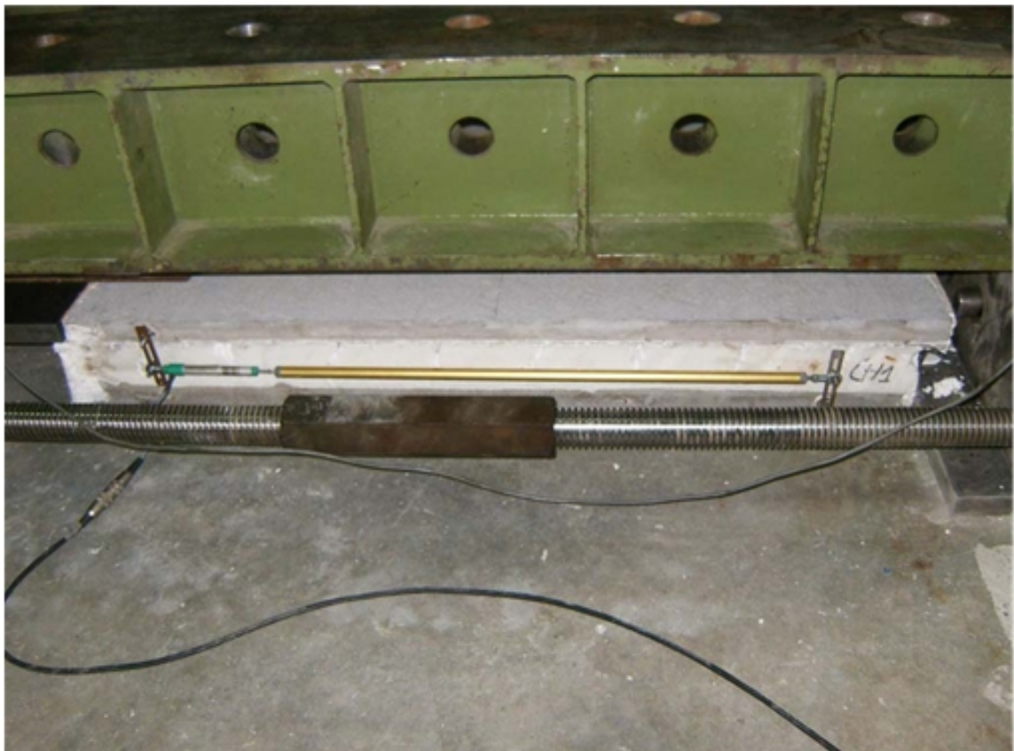
Figure 23: Sliding of the polystyrene slab
