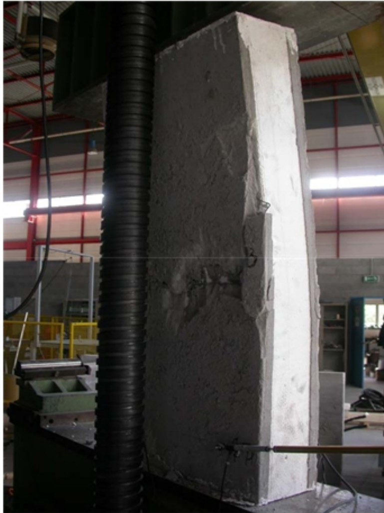
Figure 13: Breakage due to compression and flexion stresses
