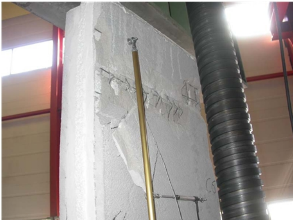
Figure 17: Destabilization of the compressed reinforcement
